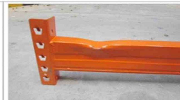
After Shear tests on beam end connectors and connector locks
