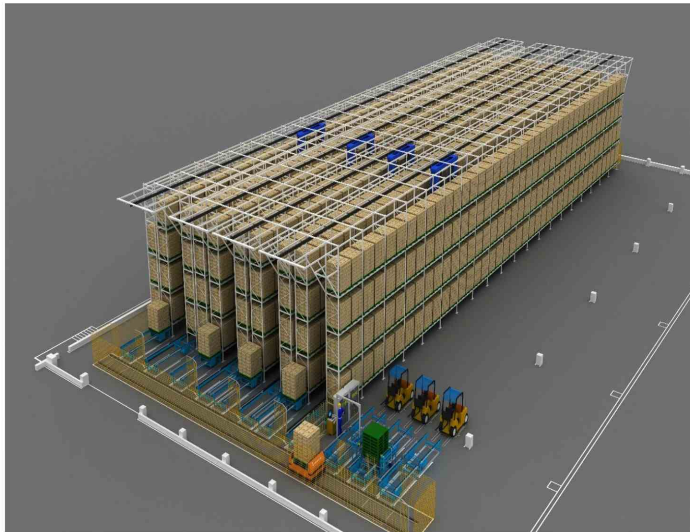
Automated warehouse ASRS system 自动化立体仓库ASRS系统
