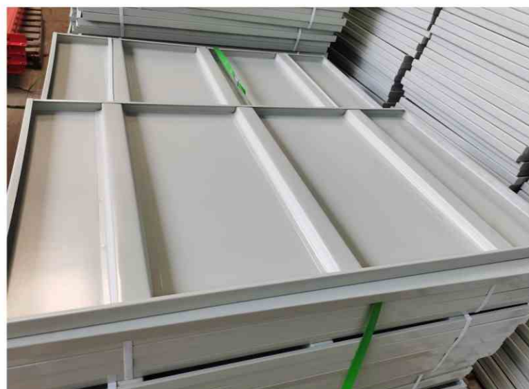
Steel decking 钢层板
