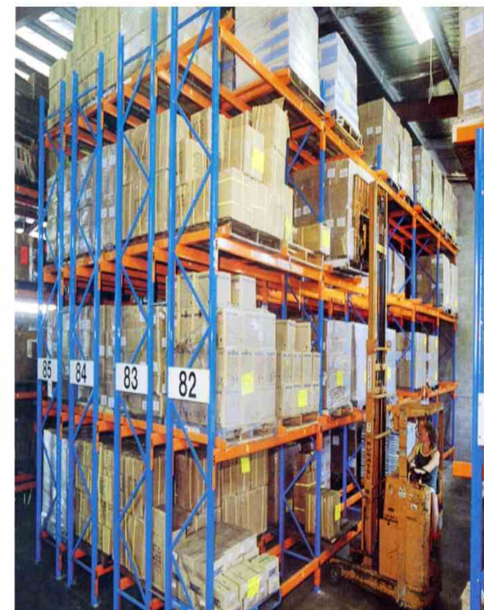
Double deep rack (with special forklift use)
