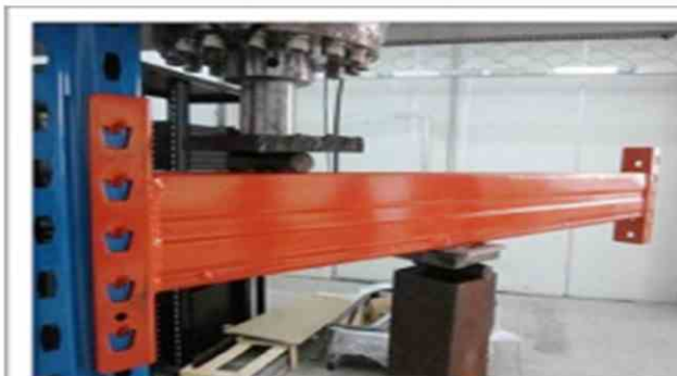
Before Shear tests on beam end connectors and connector locks
