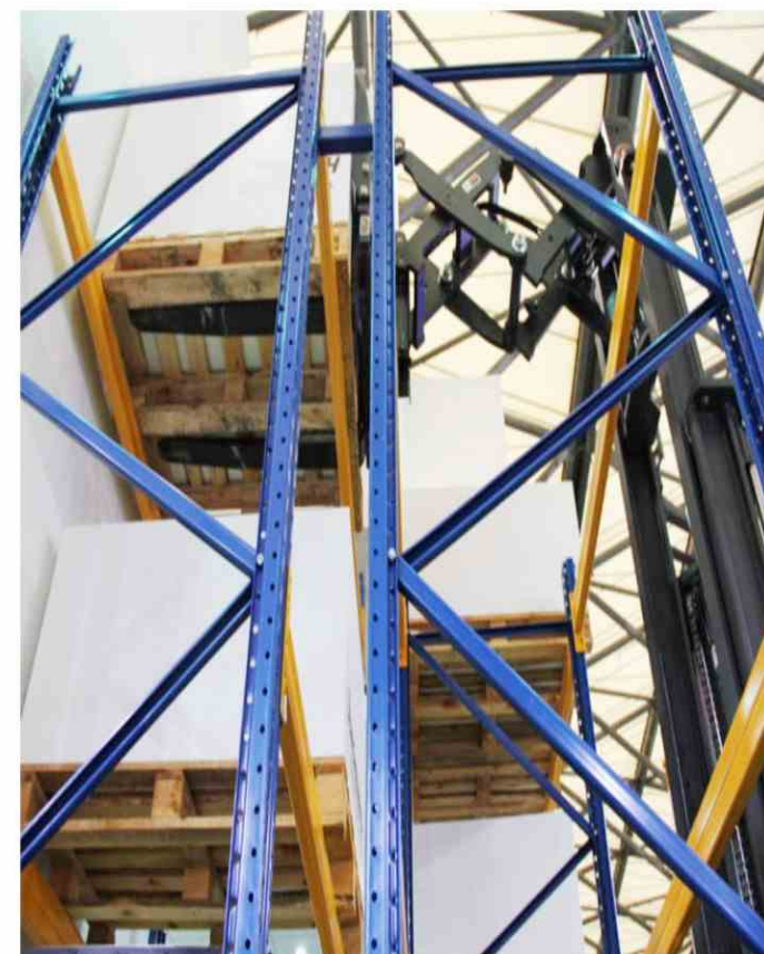
Double deep rack (with special forklift use)
