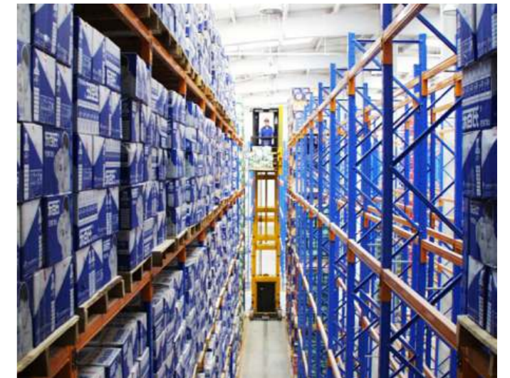
VNA rack project 窄巷式货架案例
