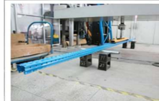
Before Bending tests on upright sections
