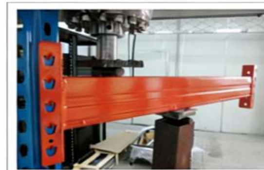
Before Shear test on beam end connectors and connector locks
