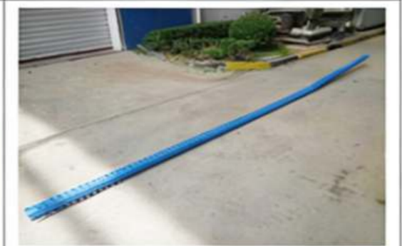
After Compression tests on uprights
