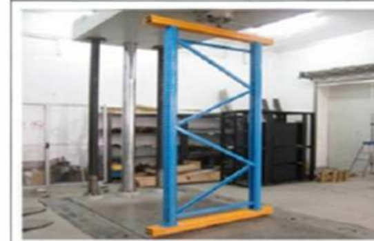
Before Compression test on uprights
