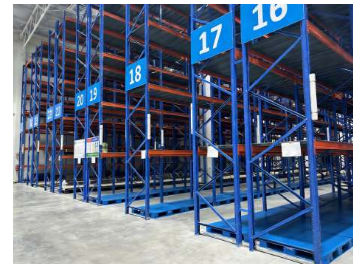
Rack with steel decking 货架铺钢层板
