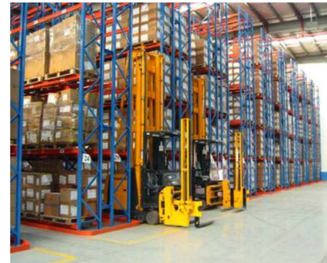
VNA rack project 窄巷式货架案例
