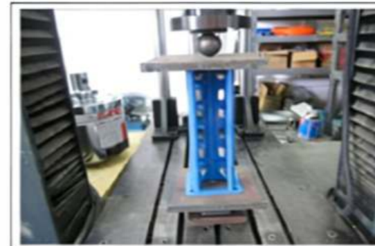
Before Stub column compression test
