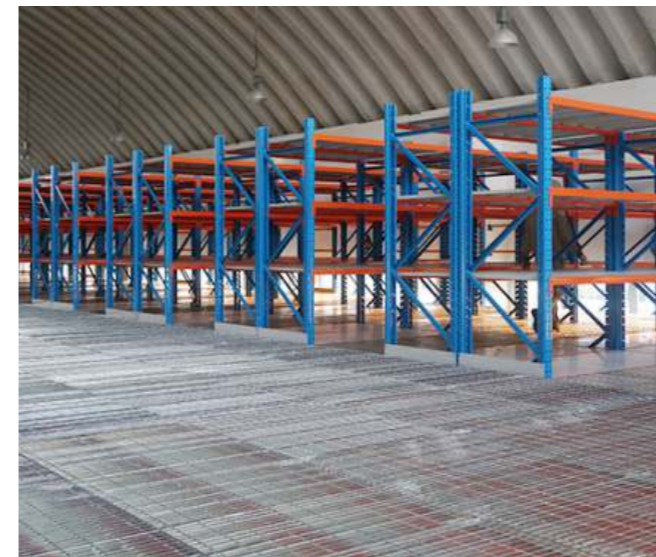
Mezzanine rack with steel grating 阁楼式货架铺钢格板
