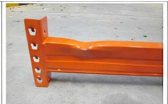
After Shear test on beam end connectors and connector locks
