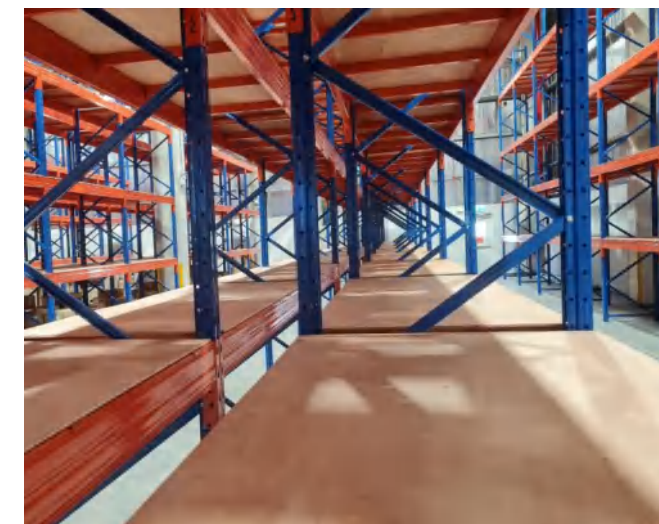
Rack with plywood 货架铺木板
