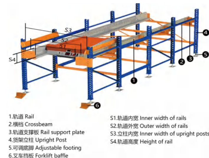
Radio shuttle rack structure details 穿梭式货架结构
