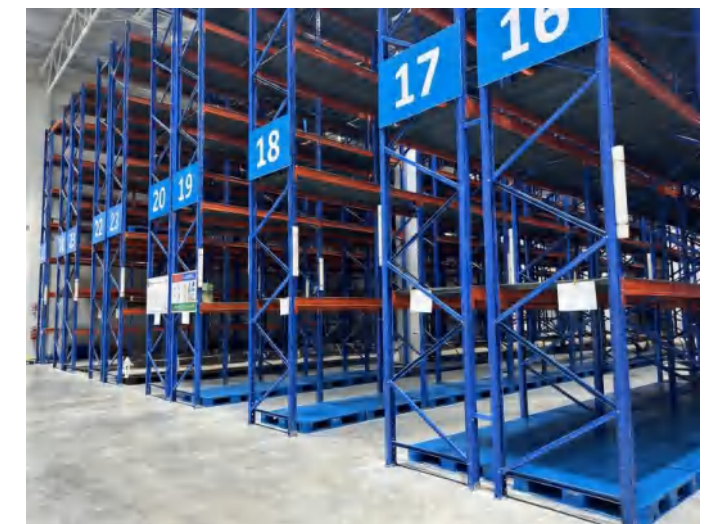
Rack with steel decking 货架铺钢层板
