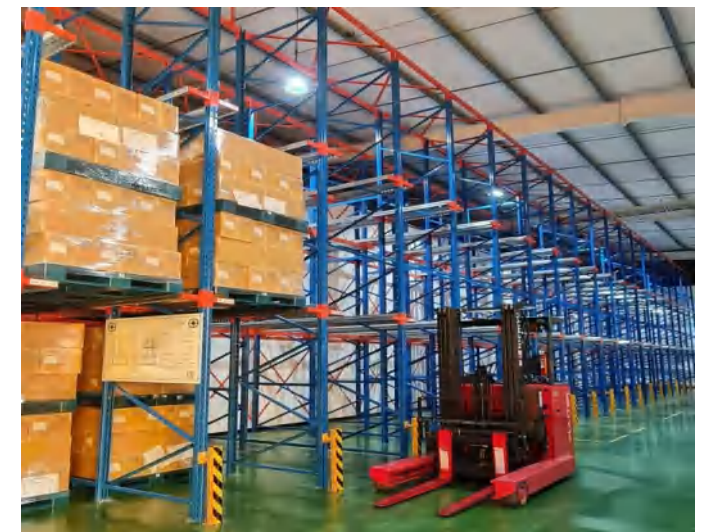
Drive-in rack project 驶入式货架案例
